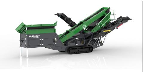
The S80 can employ the steepest screen angle of any three- way-split screening plant currently available, ensuring best-in-class screening ability in materials like sand and peastone.
