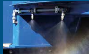
Water spraying system for dust control
