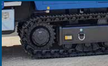
Robust tracked drives, 2 speeds, ground protection plates
