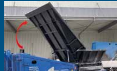
Hopper automation (FORUS) - for automatic optimisation of loading
