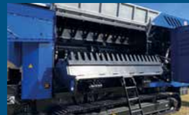
Comb door - can be opened hydraulically = free access to shredding area
