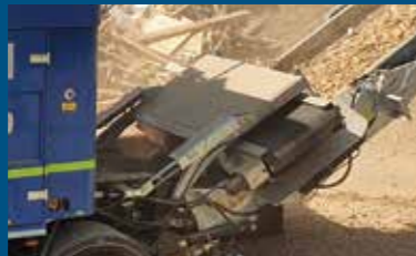
Powerful neodymium magnetic separator, hydraulically height-adjustable, metal discharge to both sides
